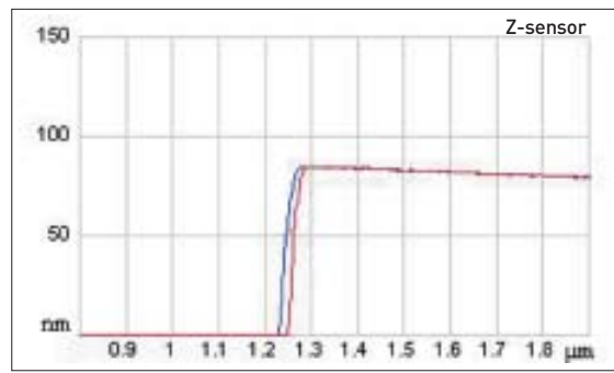
Line traces of a 200nm deep pit imaged at 12 \mu m per second tip velocity. The lack of ringing or overshoot in the line traces demonstrate the high rate of response of the Z piezo. The data trace shows piezo creep, but the Z-sensor data has no related artifact.
