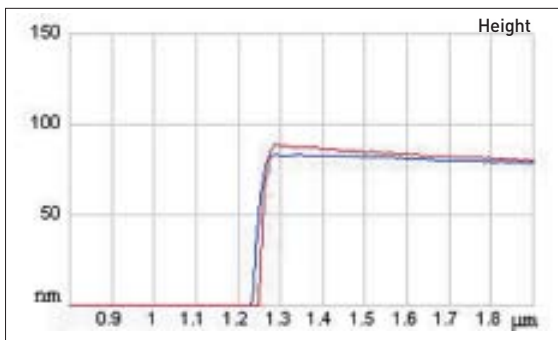
Line traces of a 200nm deep pit imaged at 12 \mu m per second tip velocity. The lack of ringing or overshoot in the line traces demonstrate the high rate of response of the Z piezo. The data trace shows piezo creep, but the Z-sensor data has no related artifact.
